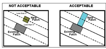
D. Remove Sections To Existing Joints
